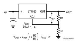
Figure 1. Basic Adjustable Regulator
