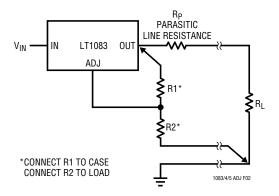
Figure 2. Connections for Best Load Regulation
