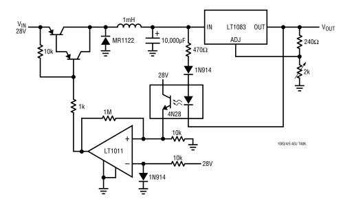
High Efficiency Regulator with Switching Preregulator
