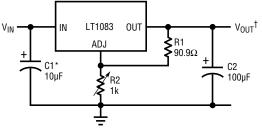
\*NEEDED IF DEVICE IS FAR FROM FILTER CAPACITORS  $^{\dagger}V_{OUT} = 1.25V \left(1 + \frac{R2}{R1}\right)$ 1083/4/5 ADJ TA08
