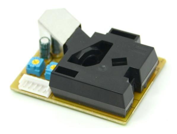
This Dust Sensor gives a good indication of the air quality in an environment by measuring the dust concentration. The Particulate Matter level (PM level) in the air is measured by counting the Low Pulse Occupancy time (LPO time) in given time unit. LPO time is proportional to PM concentration. This sensor can provide reliable data for air purifier systems; it is responsive to PM of diameter 1µm.
