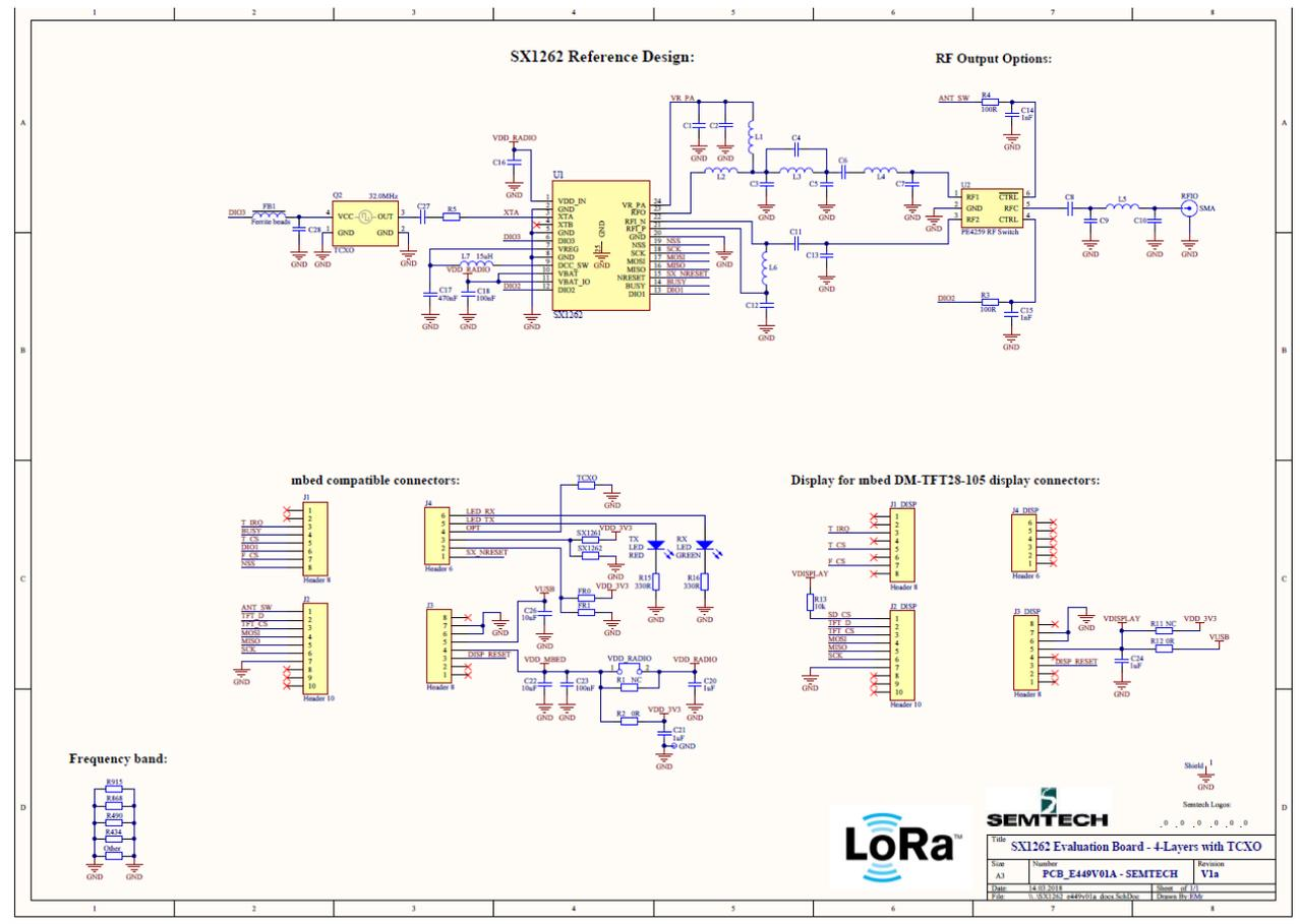
Figure 10: SX1262 Reference Design Schematic (PCB\_E449V01A)
