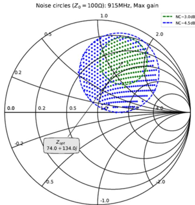
Figure 18: SX1261 Source Pull Data at 915 MHz
