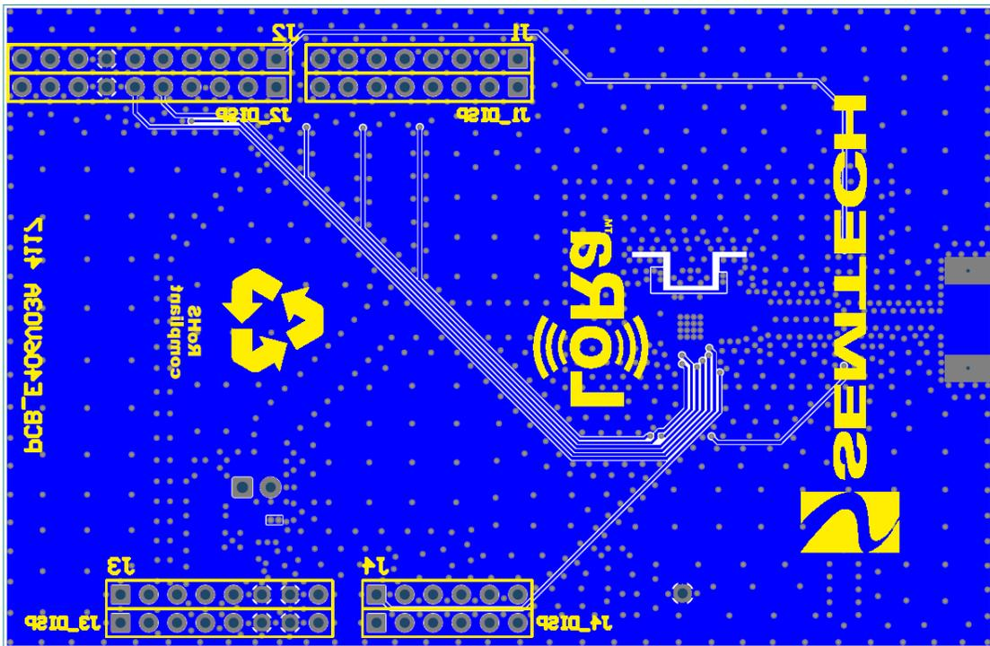
Figure 4: SX1261 Reference Design Layout – Bottom Layer (PCB\_E406V03A)
