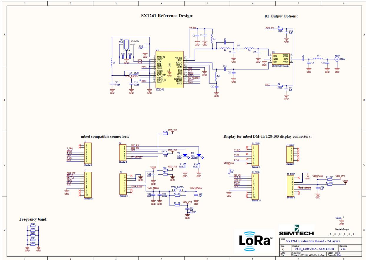
Figure 1: SX1261 Reference Design Schematic (PCB\_E406V03A)
