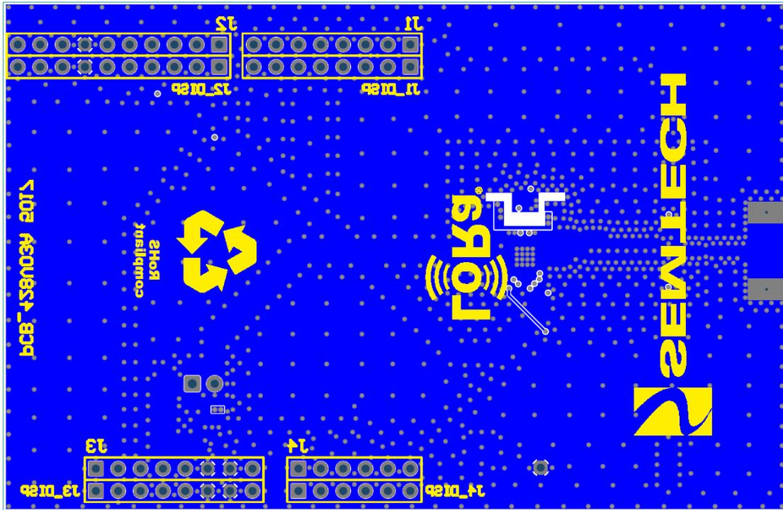
Figure 9: SX1262 Reference Design Layout – Bottom Layer (PCB\_ E428V03A)
