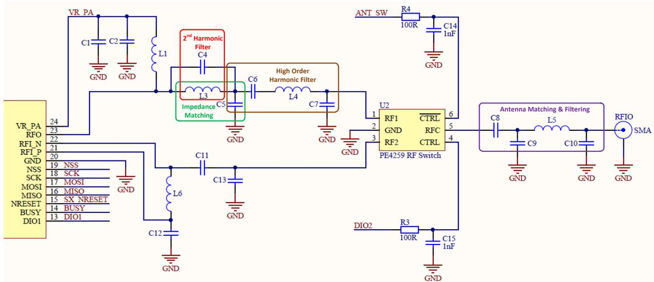
Figure 15: SX1261 Transmitter and Receiver Matching/Filtering Topologies
