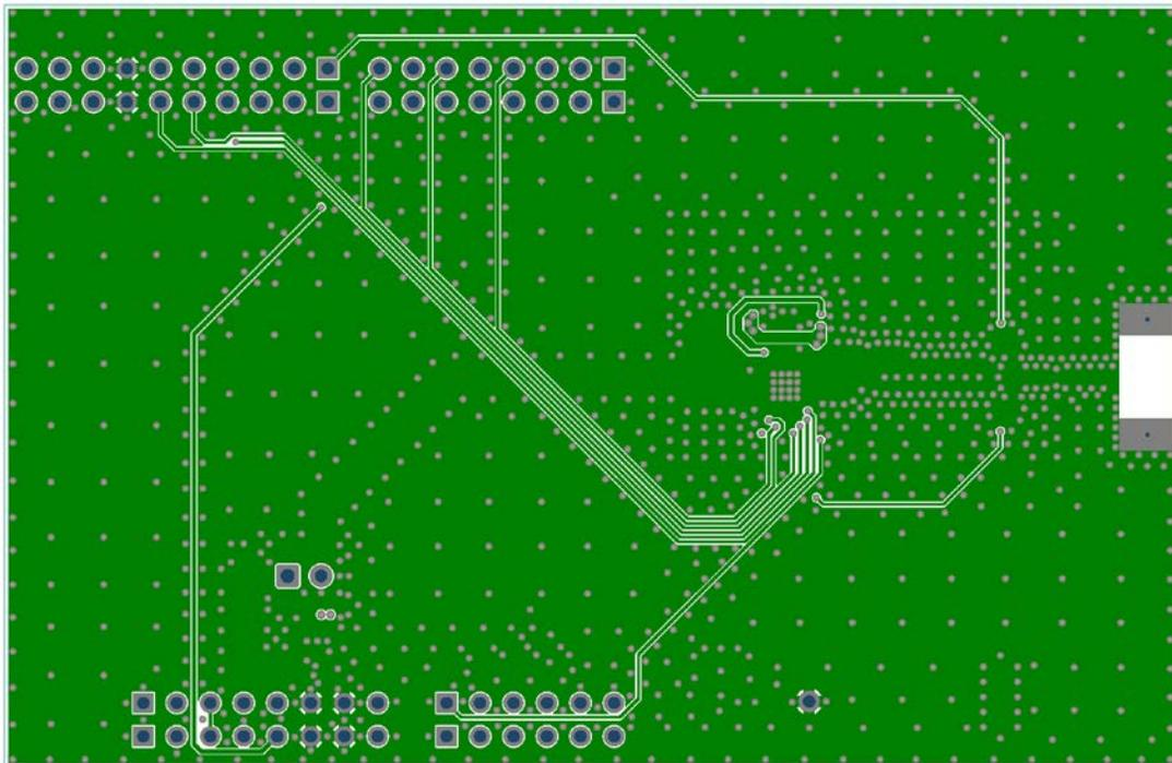
Figure 13: SX1262 Reference Design Layout – Layer 3 (PCB\_ E449V01A)
