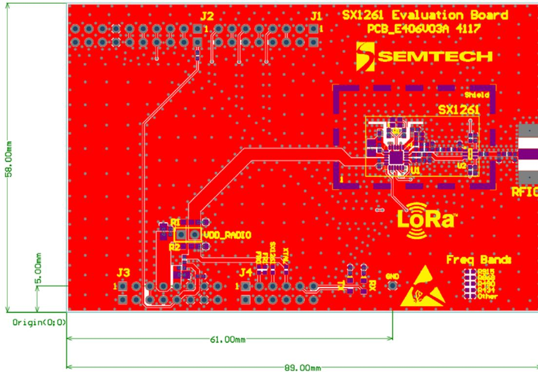
Figure 2: SX1261 Reference Design Layout – Top Layer (PCB\_E406V03A)
