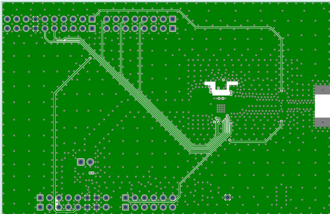
Figure 8: SX1262 Reference Design Layout – Layer 3 (PCB\_ E428V03A)
