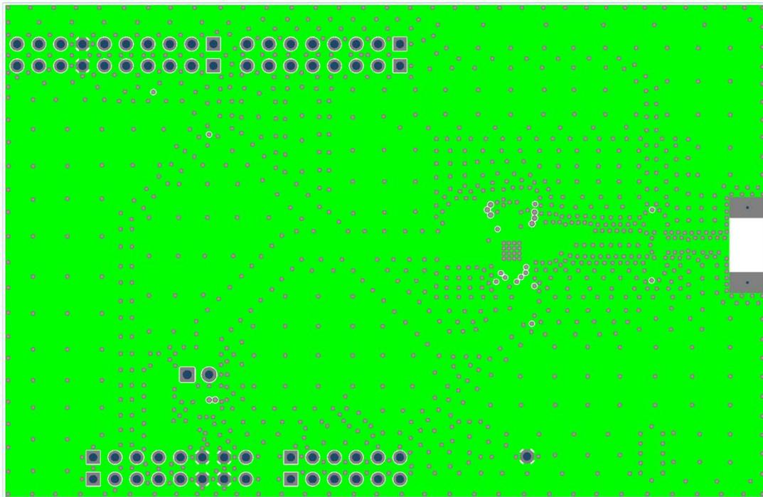
Figure 12: SX1262 Reference Design Layout – Layer 2 (PCB\_ E449V01A)
