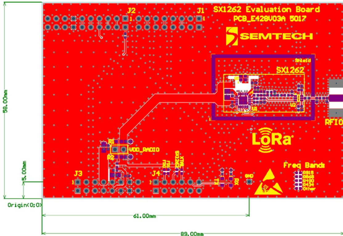
Figure 6: SX1262 Reference Design Layout – Top Layer (PCB\_E428V03A)
