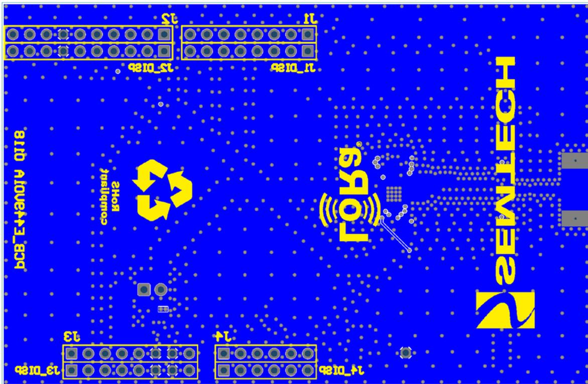
Figure 14: SX1262 Reference Design Layout – Bottom Layer (PCB\_E449V01A)
