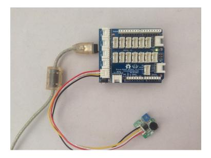
Connect Arduino/Seeeduino to PC by using a USB cable.
