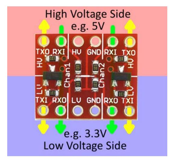
To send a signal from the low-voltage side to the high-voltage side (e.g. from 3.3V to 5V), the signal must be input at "TXI". It'll pass through the converter and come out as a higher voltage on the "TXO" (transmit output) pin.
