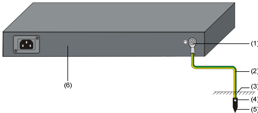
Figure 23 Ground the switch by burying the grounding conductor into the earth ground
