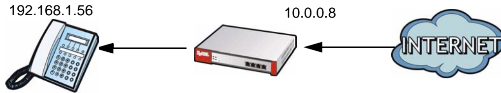
Figure 86 WAN to LAN H.323 Peer-to-peer Calls Example
